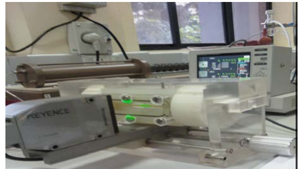
Fig.5: Arrangement for crush resistance test
