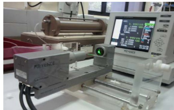
Fig.6: Arrangement for evaluating stent system compliance
